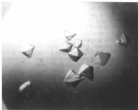
Fig. 1. Photograph of tetragonal crystals of Bowman-Birk trypsin inhibitor from barley seeds. The crystal has approximate dimensions of 0.7 × 0.4 × 0.4 mm. See the text for detailed crystallization conditions.
